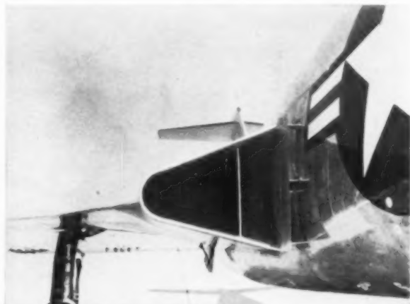
SHARP LIPS are characteristic of inlets for supersonic flight. F-101 duct intakes are triangular, with internal turning vane and boundary layer separator. Powerplants are paired P & W J57s.
